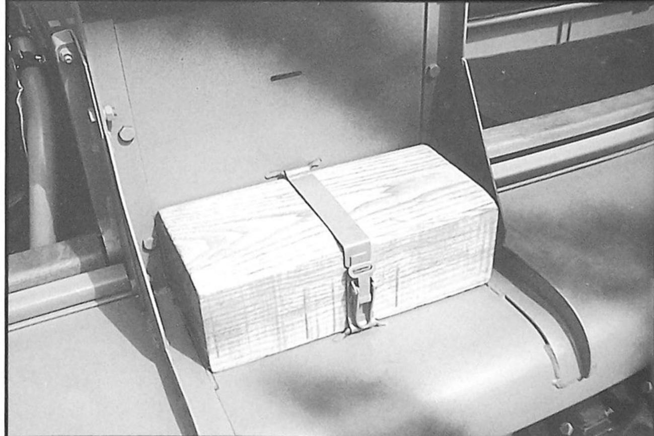
Top left: Details of the clamps securing the pick and ax. Top right: The Notek light mount on the front left fender. Note the Notek stamp on the top. Left: The first aid box mounted on the right side fender above the tracks. Above: The large wooden jack block on the left side fender above the tracks.
