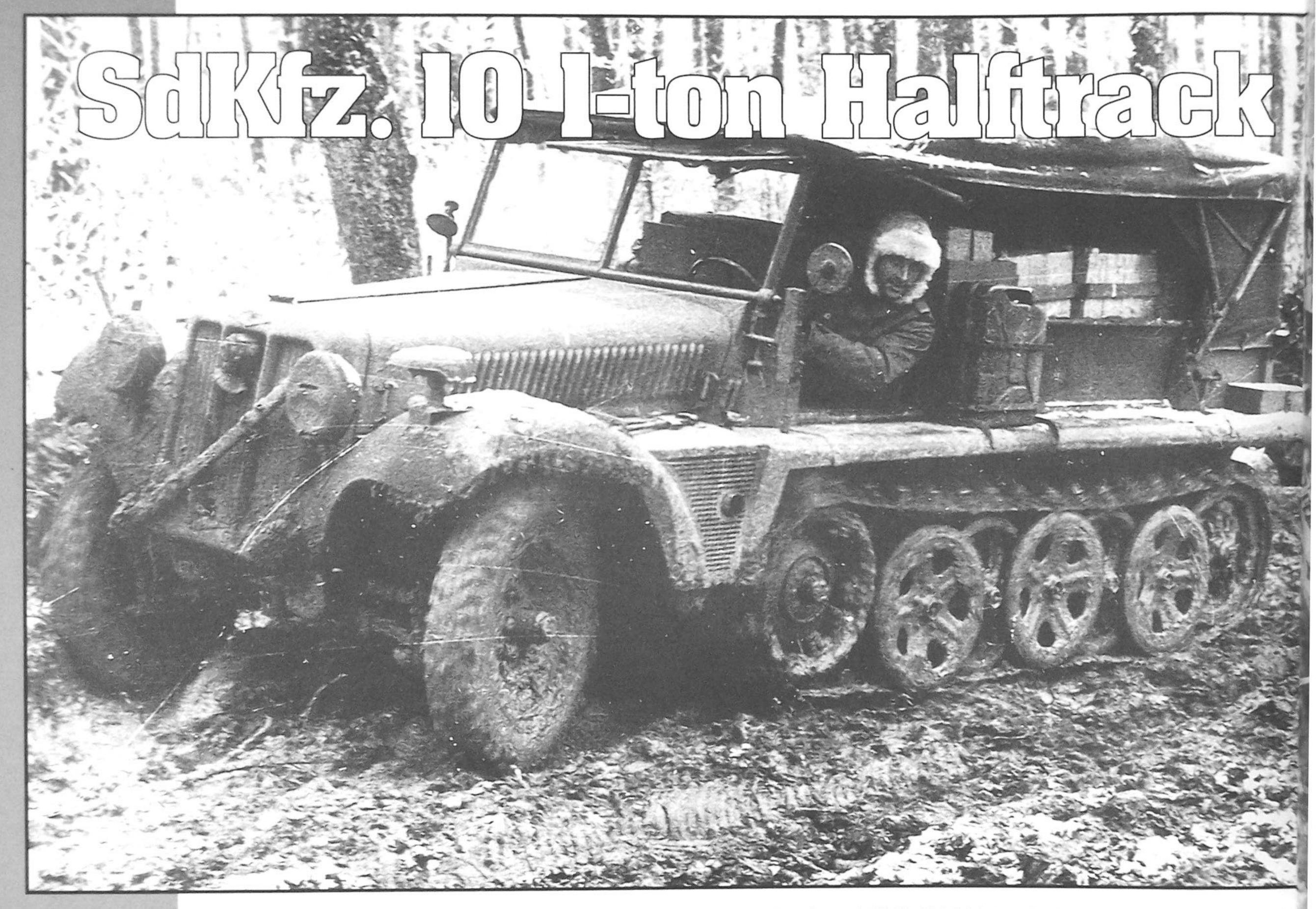
The SdKfz. 10 1-ton Halftrack was one of a number of specialized semi-tracked vehicles developed before and during the Second World War. Design of the SdKfz. 10 began as early as 1934, with several prototypes being tested. The vehicle utilized an unpowered front axle combined with a tracked rear drive composed of interleaving roadwheels and lubricated, padded tracks. The final production version of the vehicle was powered with a Maybach "NL 38" six-cylinder engine and was designated leichter
