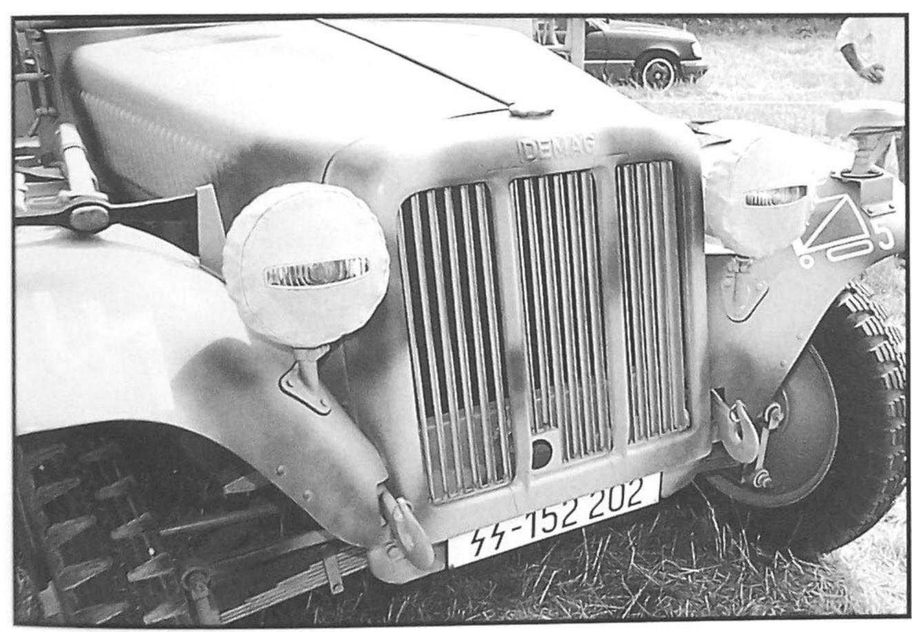
Top left: The DEMAG stamp on the radiator housing. Note the shape of the cap. Right: A close-up of the front right headlight. Note the design of the canvas cover and the amount of glass that shows though the cover. Above: An overall view of the front of the vehicle.
