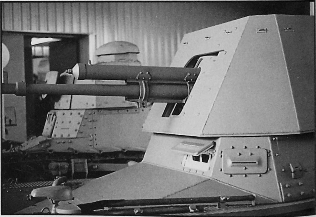
Top left, top right and left: Three views of the 4.7cm's predecessor, the 3.7cm KPUV vz. 34. It was fielded in three versions, horse-towed, motor-towed and the infantry version seen here. A modified version of this gun was installed in the 35(t) tank. Above right: The 4.7cm gun in its mount on the Panzerjäger I. (Parker)
