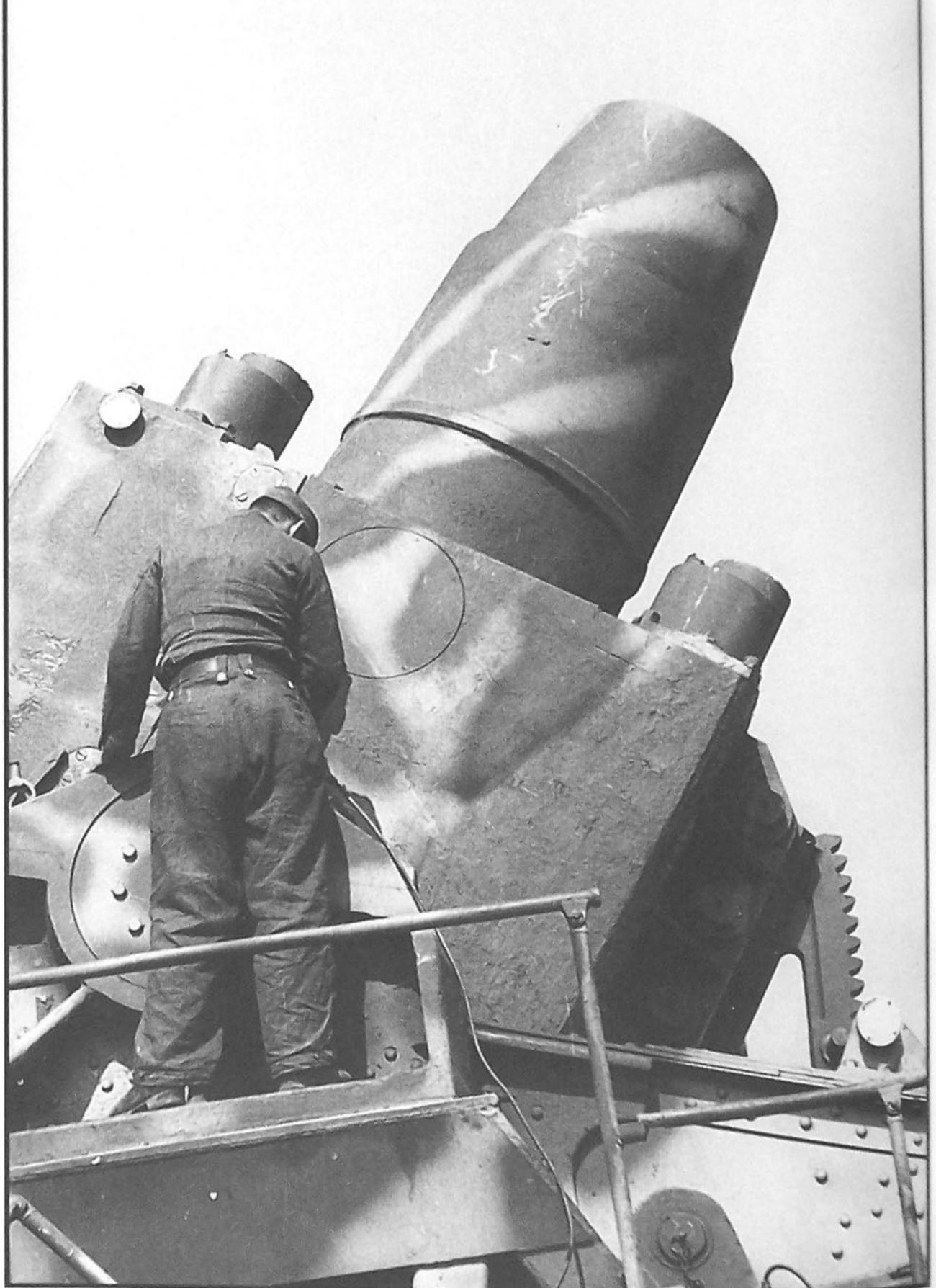
The gun tube length of the Karl-Gerät was just over five meters. The gun could elevate between 55 and 70 degrees, but could only be traversed four degrees. Larger adjustments meant moving the entire vehicle. However, using the main engine, the firing platform could be raised and lowered in only 30 seconds. A very careful and precise camouflage pattern has been applied to this gun. (BA)
