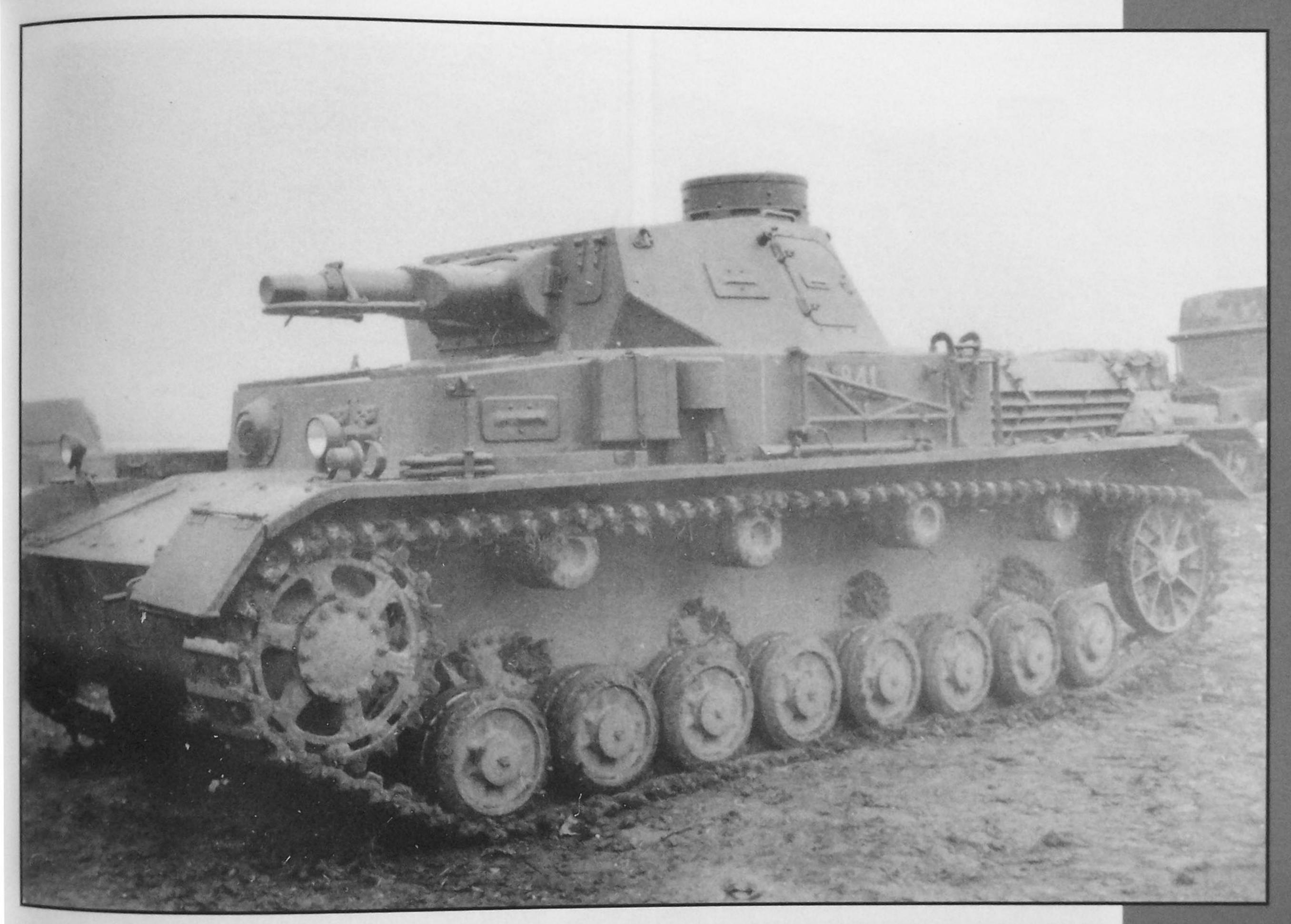
Above: An Aust. A in the 8th company, the medium company in the regiment's second battalion. Again, no further marking is visible to identify the unit. Note the deflector for the antenna rod under the gun barrel. (Photo van Berkel)
